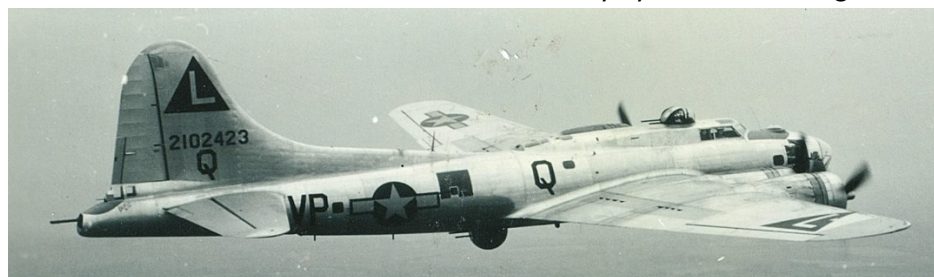
Both aircraft have the original "Stinger" tail gun position with matt olive drab anti-glare panel.
