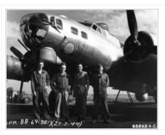
This is Sunkist Special a/c #42- 97625. You can clearly see the H2X radome in place of the ball turret. The aircraft was named after pilot James L. Tyson's California roots.
